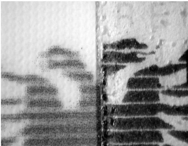
Photo replacement and seal imitation in inkjet print seen under VL mode.
