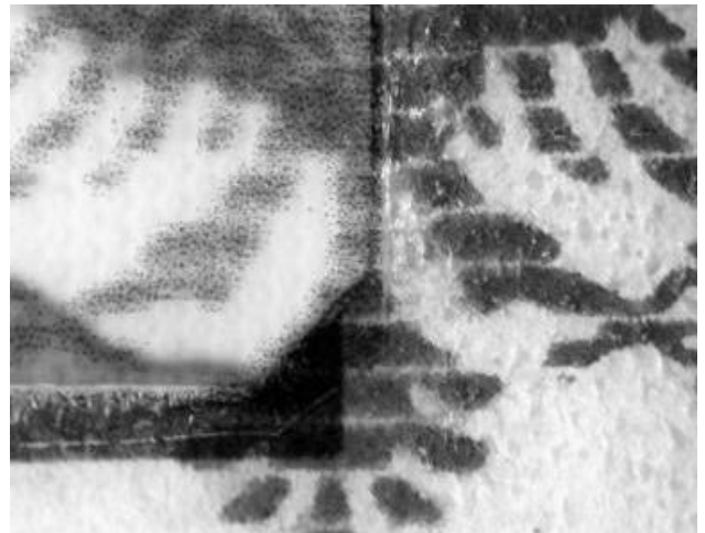
Photo replacement and seal imitation in inkjet print seen under VL mode.
