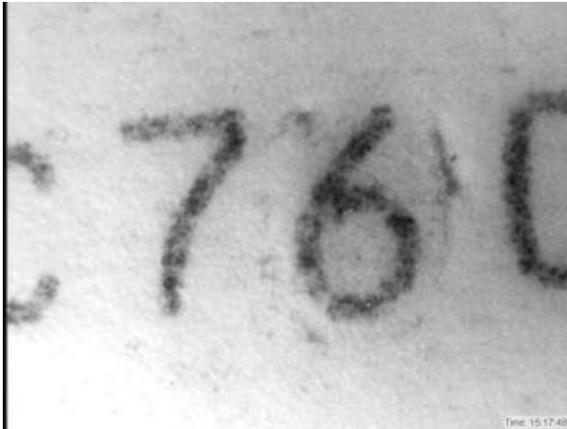
Corresponding cut and paste of single digit replaced with same material from another passport on Machine Readable area in IR mode.
