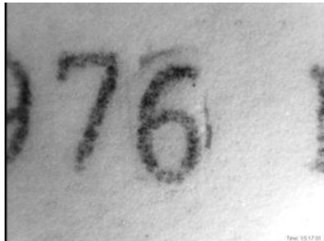
Cut and paste of single digit on birth date year replaced with same material from another passport as background design shows under VL.
