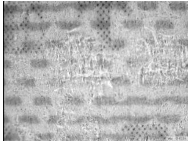
Abrasion of same area on paper surface to erase characters seen in IR mode.
